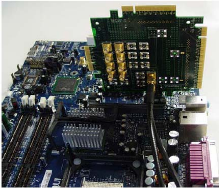
Figure 2. The compliance load board (CLB) connected to a motherboard. This fixture provides probing access for 1, 4, 8, and 16 lane connectors. This figure shows the 1 lane section being used. The SMA cables connect the D + and D - signals to the oscilloscope channels.
